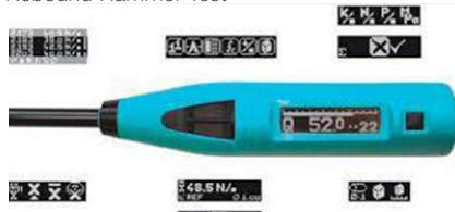
Rebound Hammer Test
