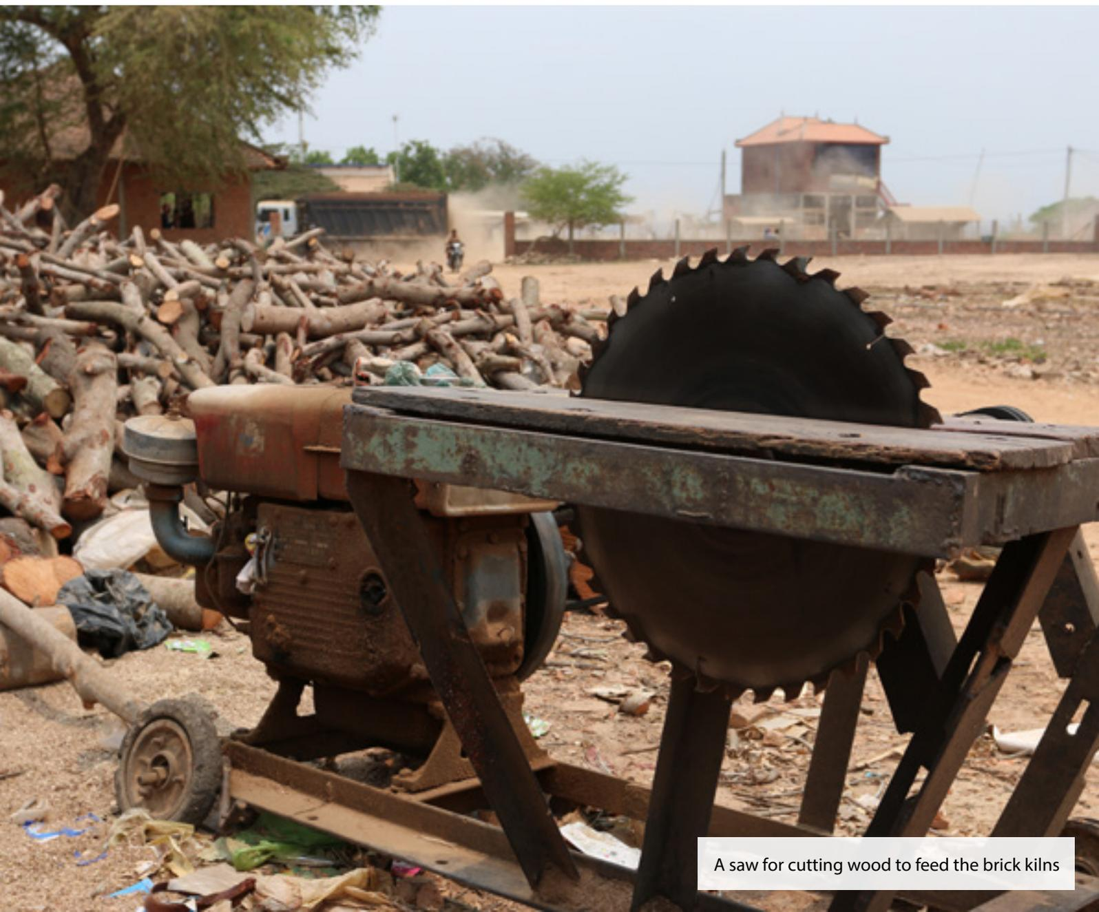
A saw for cutting wood to feed the brick kilns
